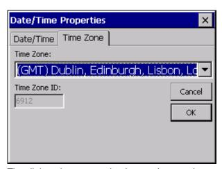
The dialog shown can also be used to set the required time zone. The «GMT» time zone is set by default, i.e. without a time shift setting. The set time zone is also retained after a restart.
